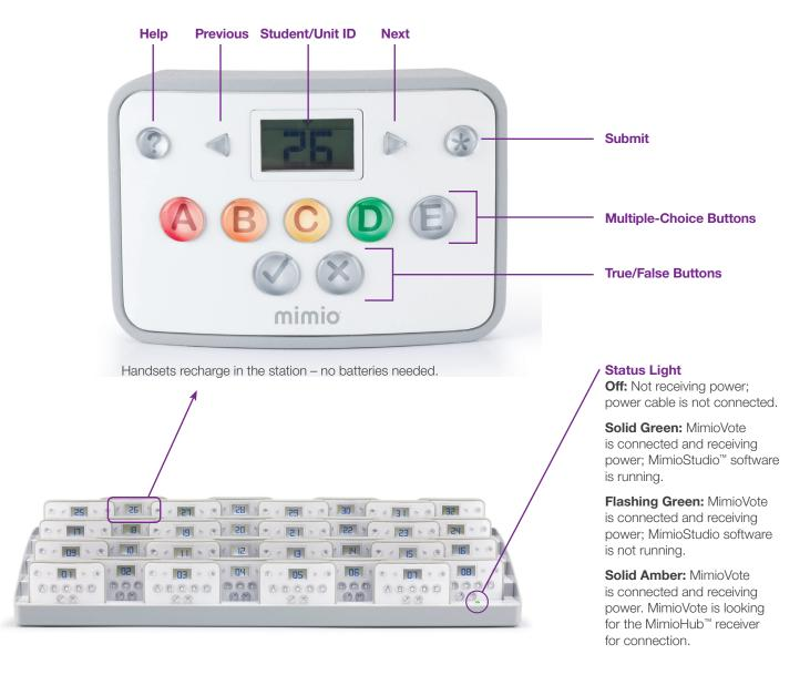
The MimioVote<sup>™</sup> assessment includes a charging station that also stores all of your MimioVote units. You can place any unit into any slot on the station, and it will automatically be assigned the number for that slot. No need to match a particular unit to a particular slot!
