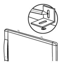
16. Remove the L-brackets and drill a hole at each mark using a ¼ in (6.35 mm) drill bit.
