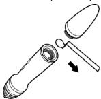
3. Replace the top onto the body of the stylus and turn clockwise to attach.
