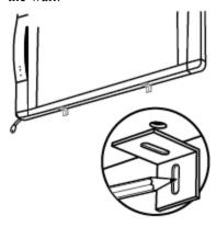
12. Remove the L-brackets and drill a hole at each mark using a ¼ in (6.35 mm) drill bit.
