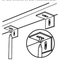
c. Using a screw driver and a #10x2½ in (M5x60mm) screw, securely fasten each bracket to the wall.
