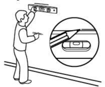
3. Align the mounting bar with the horizontal line and make a mark on the wall in the center of four of the holes in the mounting bar.
