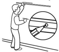
4. Drill a hole at each mark using a ¼ in (6.35 mm) drill bit.
