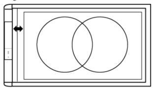
2. Click the stylus anywhere on the MimioBoard surface. Interactive mode starts and the calibration screen appears.
