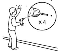
5. Insert a drywall anchor into each of the four holes so that each anchor is flush with the surface of the wall.
